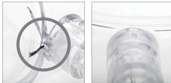
Figure 1 Medical device housing after exposure to Virex TB
