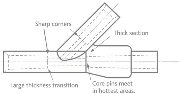
Figure 2 shows a Y-site design that suffers not only from thick sections and sharp corners but also from thin areas. These thin areas will serve as flow restrictors and will make it difficult to fill and pack out the part properly.
