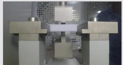
Unload the samples and run a reverse side impact test on the exposed and control samples
