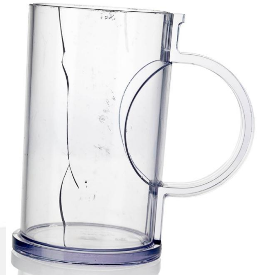
SAN after 30 cycles and drop test
