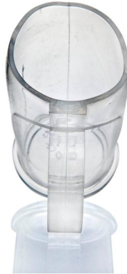
Methacrylate styrene after 50 dishwasher cycles and drop test
