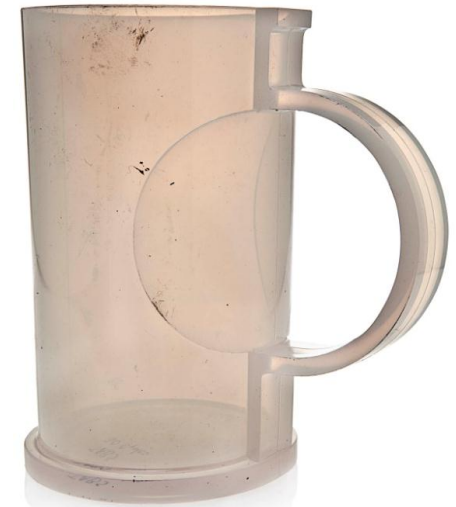
TABS after 30 dishwasher cycles and no drop test
