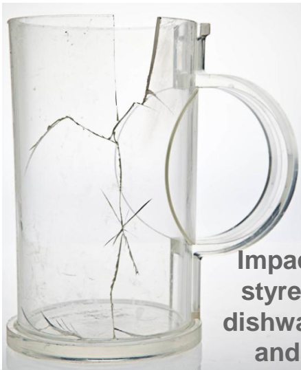
Acrylic after 75 dishwasher cycles and drop test
