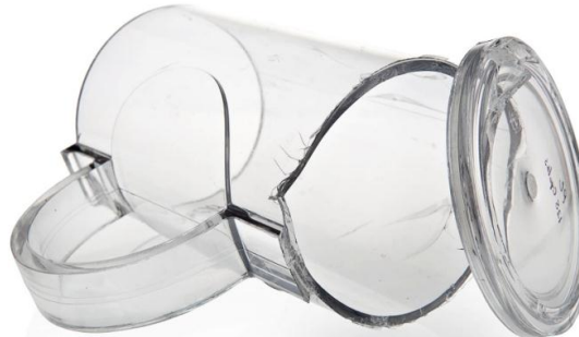
Polycarbonate after 125 dishwasher cycles and no drop test
