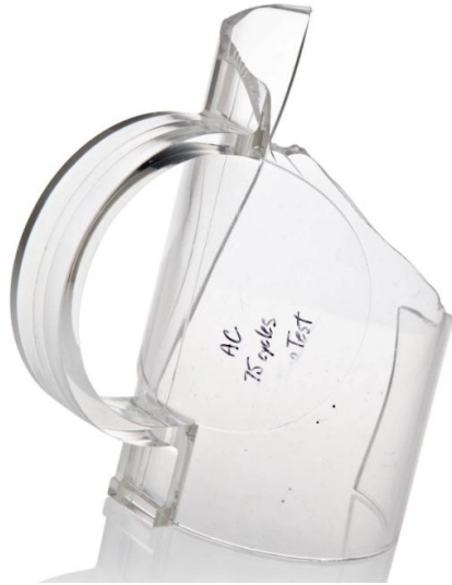
Acrylic after 75 dishwasher cycles and drop test
